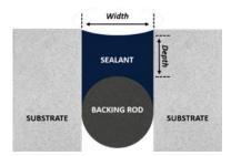
Wider joints can accommodate more total movement than narrow joints.
